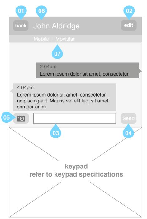
Wireframe illustrating an SMS message thread:
