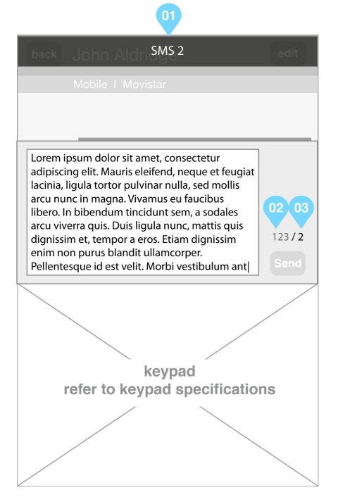
Wireframe illustrating the composing of an SMS message when the message to be sent comprises of multiple SMS packets
