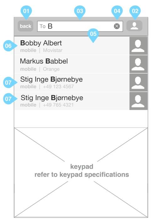
Wireframe illustrating an SMS contact search autocomplete
